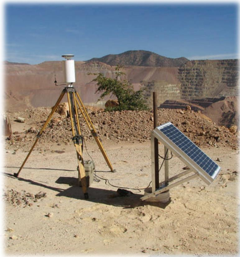
Since 2000, **Orion Monitoring Systems, Inc.** has designed and implemented GPS field stations for tall building, bridge, dam, landslide, slope and tectonic deformation monitoring. Our latest offering, **CAN-GPS**, compresses our traditional integrated systems into the smallest, lightest package yet.
